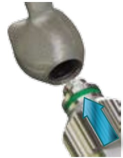
Insert appropriate diameter Reamer into the casting.
